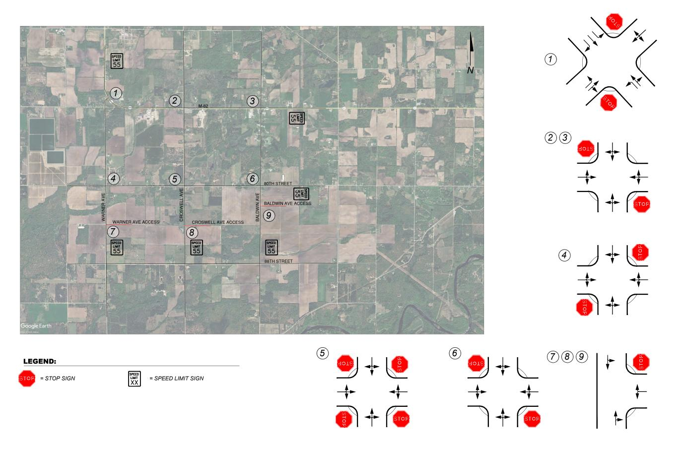
Figure 5: Proposed Lane Configurations / Traffic Control
