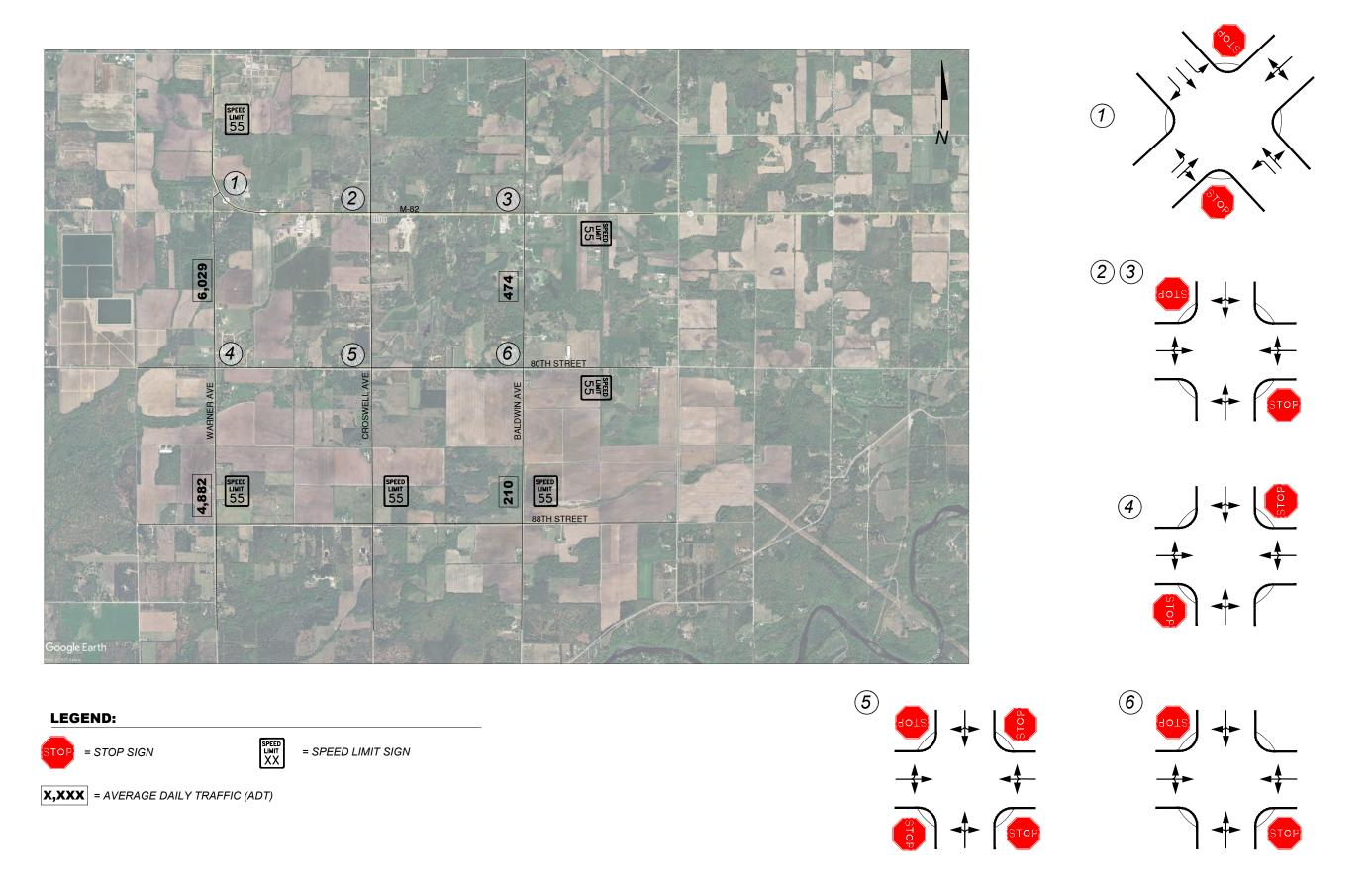
Figure 3: Existing Lane Configurations / Traffic Control
